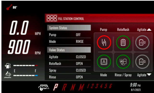
3 in Fill Rinse Pump OFF:
