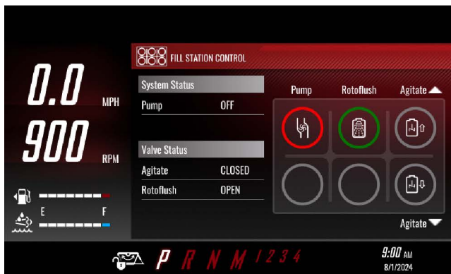
2 in Fill Rotoflush Pump OFF:
