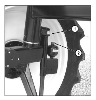
*NOTICE: If oil comes out of the accumulator charge port, the accumulator has failed. Contact your dealer for a replacement accumulator.*
