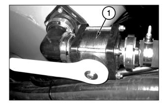
Remove the cap from the product quick fill inlet (1) and connect the hose from the nurse tank to the inlet.
