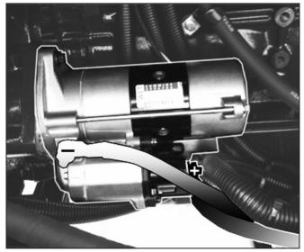
*NOTICE:* NEVER continuously crank the starter more than 30 seconds. Stop cranking and allow the starter to cool for 2 minutes between cranking to avoid damaging the starter.
