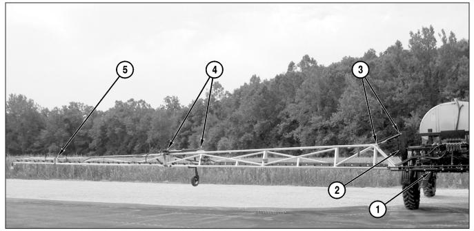
The Pommier boom is equipped with five sets of grease fittings. Apply an ample amount of lithium grease through each of the grease fittings.
