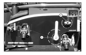
The product strainer (1) features 50 mesh screens, which should be checked and cleaned after every 50 hours of operation or as needed.
