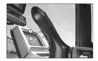
NOTE: The joystick will not shift the transmission into NEUTRAL. To obtain NEUTRAL from a REVERSE gear, release the bottom trigger button (2) on the joystick.
