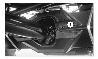
The other two slip joint grease fittings (1) are located under the Apache Sprayer, between the differential and each drop box U-joint.
