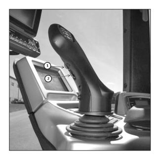
NOTE: The joystick will not shift the transmission into NEUTRAL. To obtain NEUTRAL from a FORWARD gear, squeeze either trigger button (1 or 2) on the joystick.
