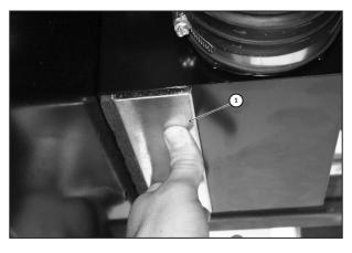
Insert the new filter into the frame with the air-flow arrow pointing toward the A/C box.
