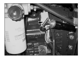
Check the transmission fluid level with the transmission fluid at normal operating temperature, transmission in NEUTRAL position, and the engine off.
